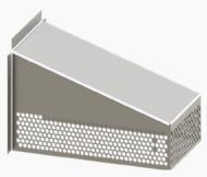
If the pump is not supplied with enough water, it will run dry. As a result, unhealthy operation and malfunctions are inevitable. The main purpose of Antivortexhood is to protect the circulation pump against dry running and cavitation.
