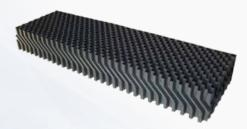
The drift eliminator used in the RTCY series prevent the process water from leaving the circuit by air, up to 0.02% of the cycle water. This reduces water and chemical consumption. It is very light as it is made of PVC material. In this way, the water distribution system can be easily disassembled in case of maintenance.
