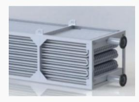
RTCY series tower coils will be manufactured from high quality steel pipes with hydrostatic test and are subjected to hot dip galvanizing process after manufacturing. At the same time, we have stainless steel applications depending on the request of our customers. The coils are placed horizontally in the tower and are tested with 10 bar compressed air in the test pool.
